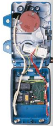
42570-1 Tristate control (DC-Com & DC-Pro)
