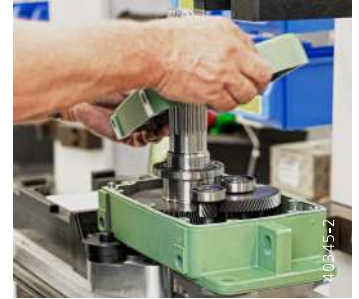
The DC-II gearbox is still manufactured in-house by Demag. This is the only way for us to meet our demanding quality requirement for the chain hoist.
